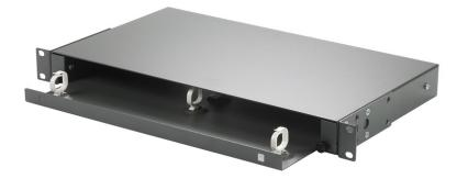
These 1RU and 2 RU fibre storage tray allows excess optical fibre cord/s to be stored into coils or loops. The half slide out storage tray is either 19 or 21-inch rack mountable. Using 4 x M6 mounting screws and cage nuts supplied. The tray is vented to allow cooling air stream to flow in the rack. It is recommended individual coils of optical fibre cord be secured by several hook and lop style ties. The 1RU can store up to 10M of 5mm diameter cord and the 2 RU unit up to 20m of the same cable.
